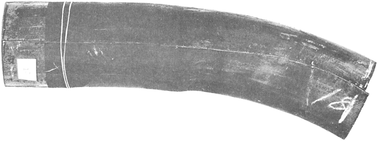
Figure 12-23.—Tube fold (fabrication defect).
