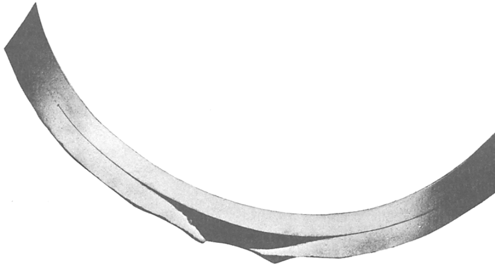
Figure 12-22.—Lamination of a tube wall (fabrication defect).
